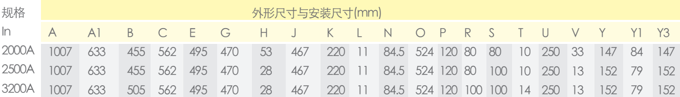
EXATC-PC-2000A~3200A外形安装尺寸图
