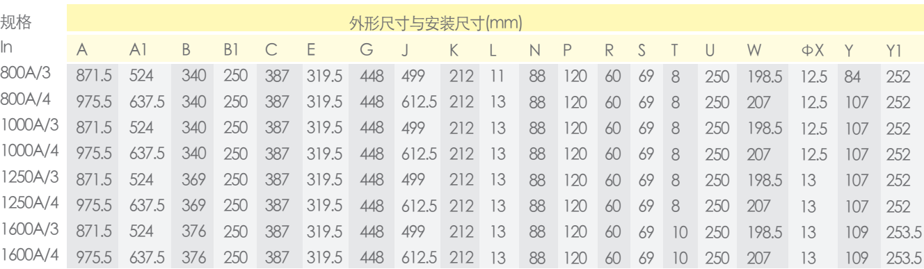
EXATC-PC-800A~1600A外形安装尺寸图
